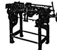
PETERS JUNIOR CARTON FOLDING AND CLOSING MACHINE closes 35-40 cartons per min., no operator.
